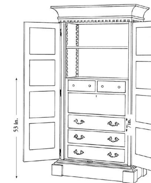
ST / DW (Standard / Drawers) W x D x H 45.5 in. x 22.5 in. x 90 in. 115.5 cm. x 57 cm. x 228.5 cm. (Interior Depth: 17 in. / 43 cm.) (Interior Width: 35 in. / 89 cm.)
