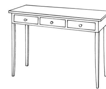
DP / ST (Deep / Standard) W x D x H 43 in. x 23 in. x 30 in. 109 cm. x 58 cm. x 76 cm.
