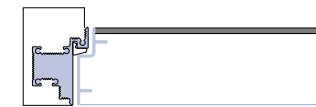
Ribasso (da 1 a 4 mm) - lato a spingere / Push side lowered (from 1 to 4 mm)
