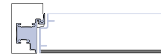
Ribasso (da 1 a 4 mm) - lato a tirare / Pull side lowered (from 1 to 4 mm)
