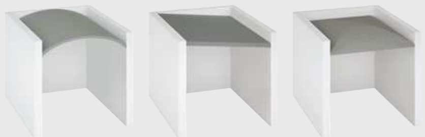
Volta a botte. Barrel vaulted ceiling.
