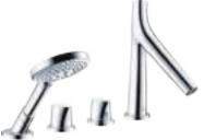
/ maximum pull-out length of hand shower: 1.10 m / maximum flow rate at 3 bar: 18 l/min / flow rate for bath spout at 3 bar: 18 l/min / flow rate of hand shower at 3 bar: 16 l/min / min. operating pressure: 1 bar / max. operating pressure: 10 bar / Safety stop at 40 °C
