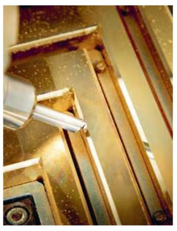
A diamond is used to mill the beveled chamfer at an angle of exactly 45° to a high gloss.
