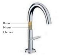
Chrome is the standard surface in the sanitary environment and has proven itself in the bathroom over many decades. Through the electrochemical deposition of various metals, and depending on the type of substrate, a copper layer is built up in the electroplating bath, followed by a bright nickel and chrome layer on the basic brass body.
